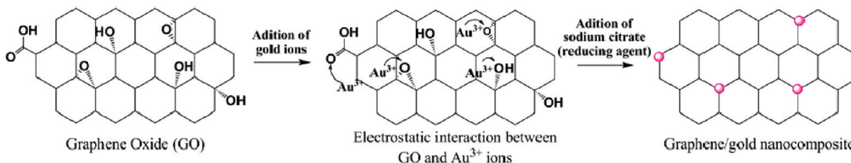
Figure 9. Schematic representation of the mechanism of nucleation of gold nanoparticles at functionalized graphene surface.
